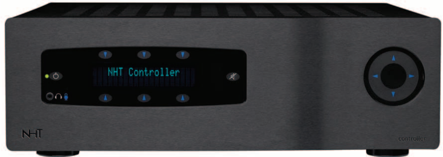
NHT Controller with its multi-talented touch-screen panel (left) and touch-wheel volume and navigator (right). The display was readable from across the room and that greatly enhanced the efficacy of the remote control.
